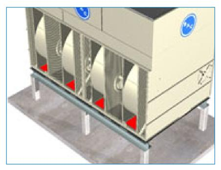
Solid bottom panels are required when the unit is installed elevated by 30 cm or more and when intake air is ducted to the unit.
