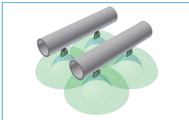
Nozzle spray distribution type for condenser
