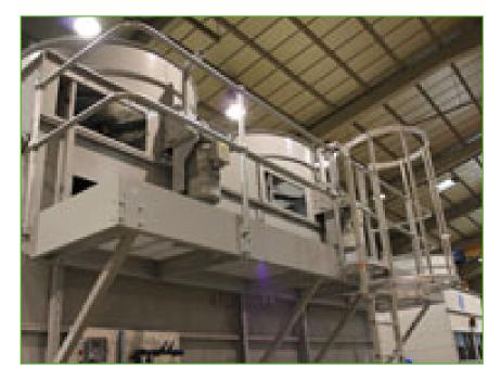
**Platforms, a ladder, safety cage and handrails** facilitate **easier and safer access** to the unit, making inspection and maintenance easier and conforming to European safety standards.
