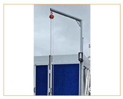
With the motor removal davit, lowering or lifting your motor from/onto the unit top is easy!
