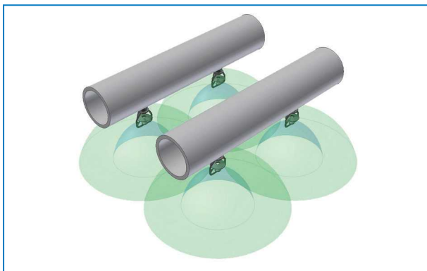
Nozzle spray distribution type for closed circuit cooling tower
