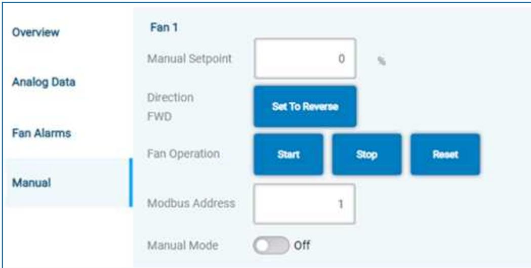
The Modbus address is only available for a specific fan, not when you have selected "All Fans". Set manual mode to "off", if normal operation needs to be resumed.
